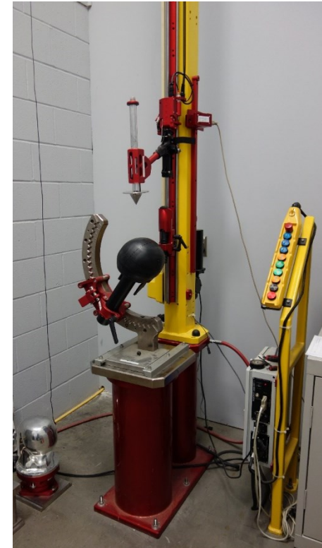
IN-HOUSE CSA TESTING: HARD HAT PENETRATION
